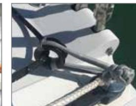
LOOP® Reefthimble installed as a deflector
