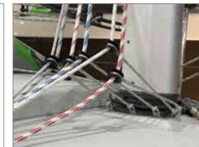
LOOP® Strops to adjust the right height for halyard deflection
