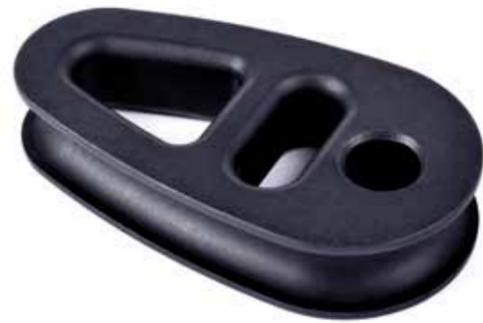
We developed a set of new Thimbles for Furling rope and other applications. KOHLHOFF LOOP® Furling Thimbles are made of high quality black anodized alloy. They have a straight pin hole and fit most common jaws of furling units. The lashing eye is smooth and round and designed to accommodate sufficient lashing to securely fasten the tack of the sail. Available in four different sizes from 9 to 15 mm rope diameter.
