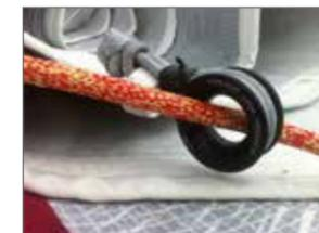
LOOP® Reefthimble installed at the luff of a mainsail
