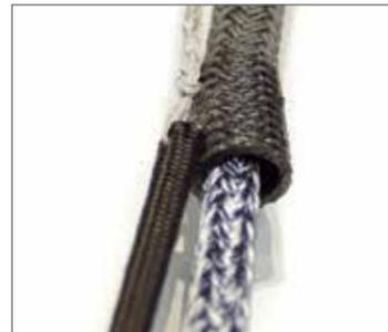
The locking cover is working like a single braid splice.
